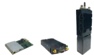
NBMesh-4Watts Module/Airborne/Handheld(Double Antenna) (Digital microphone, location/electronic map, RJ232/485/422, RJ45)
